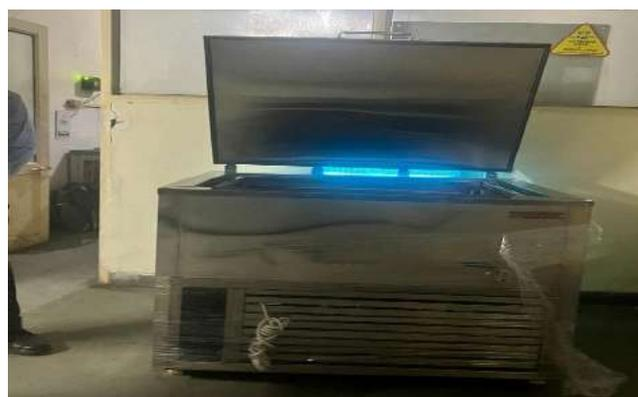
*Kulfi-making Machine at Experimental Dairy Plan*
