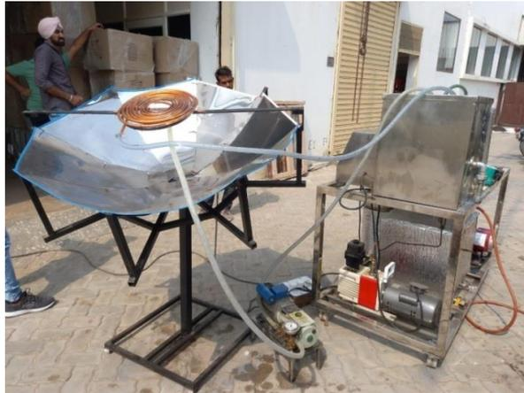
**Solar-Thermal fluids driven hybridized Ice bank tank for milk cooling**
